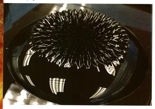
The science of ferrofluid will first be introduced. Ferrofluid is a liquid containing numerous tiny magnets that can change its shape under the influence of magnetic field. The physical properties of ferrofluid and the applications based on these properties will be discussed.
