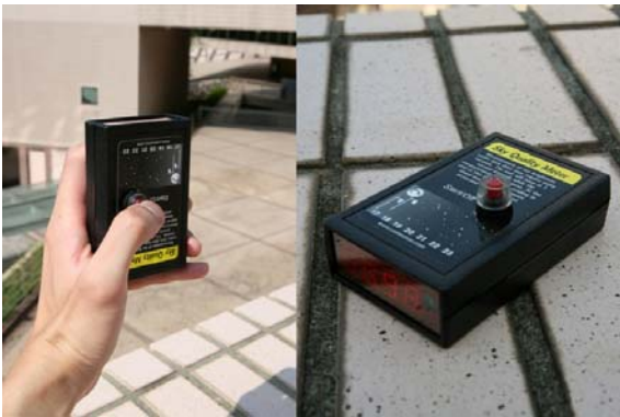
Image 3: 36 Sky Quality Meters were distributed to 200 secondary school students, campsite staff, and astronomy enthusiasts to measure the night sky brightness at multiple sites in Hong Kong for 15 months.
