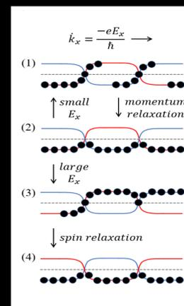
Left: Schematic illustration of the effect of electrical field in the momentum space. Bottom: Initial and final state of the electrical switching
