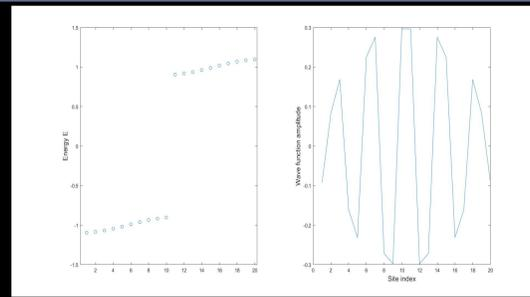
Fig.2 Energy levels and wave function of the finite chain with 20 sites. The first panel is plotted with  $v=0.1$ ,  $w=1$ . The red circles denote the edge states, and its corresponding wave function amplitude on the chain is plotted, which is localized at the two end of the chain. The second panel is plotted with  $v=1$ ,  $w=0.1$ . There are no edge states, and a typical wave function is plotted, which shows no localization
