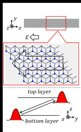
Set up: A ribbon is placed along the  $x$  direction while an electric field is also applied along this direction. As demonstrated, the electron wave packet would experience oscillation along the transverse direction
