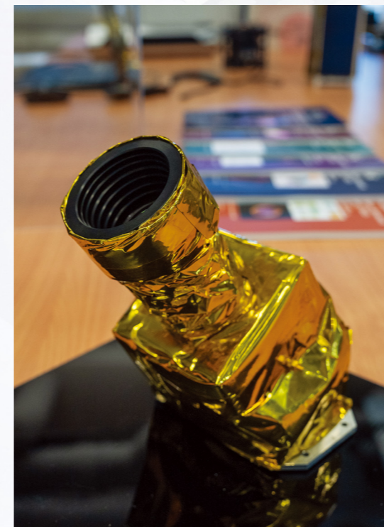
The ILO-C small wide-field telescope, developed by HKU LSR and ILOA, will capture images of the Galactic plane from the Moon on the Chang'e-7 mission.
