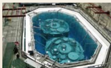
The first pair of antineutrino detectors, 5m tall by 5m diameter each, submerged in pure water inside the Daya Bay Near Hall.
