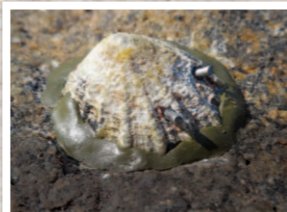
An example of the Robolimpet - a temperature datalogger
