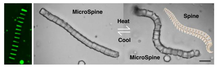
Microscale spine-mimicking structure, MicroSpine, has been created via colloidal assembly of soft and hard components, which can change shape by controlling temperature and can be utilised for cargo encapsulation and delivery. Image Credit: Dengping Lyu
