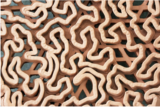
Image 4: A 3D designed reef tile was printed through a robotic 3D clay printing method with generic terracotta clay and then fired at 1125 degrees Celsius. (Photo credit: Christian J. Lange)
