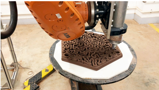
Image 6: A 3D designed reef tile was printed through a robotic 3D clay printing method with generic terracotta clay and then fired at 1125 degrees Celsius. (Photo credit: Christian J. Lange)
