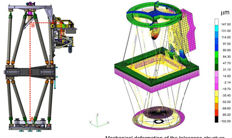
$\Delta T = 30^{\circ}C$ : Expansion between A and F = 150µm. Change of the focal plane of 5µm for a temperature variation of 1°C
