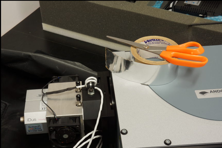
The InGaAs camera, showing additional cooling fans.
