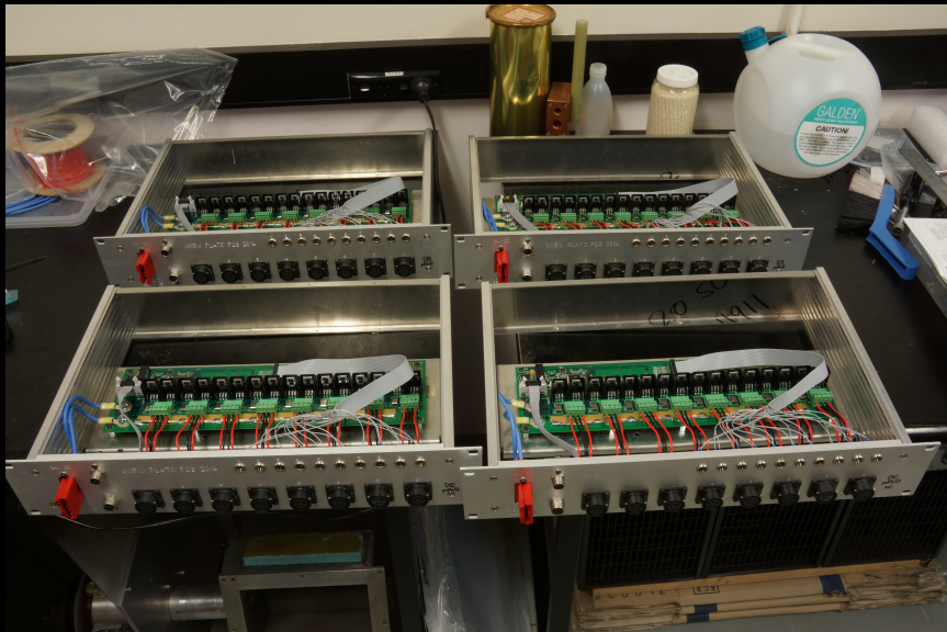
New 24VDC Power Distribution Boxes for Dome A, 2015.
